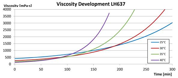
Measuring conditions: Rheometer, CP50-1, measuring gap 0.1mm
