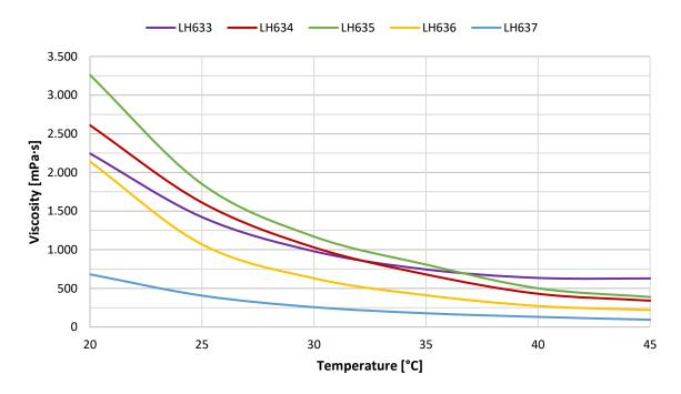
Measuring conditions: Rheometer, CP50-1, measuring gap 0.1mm
