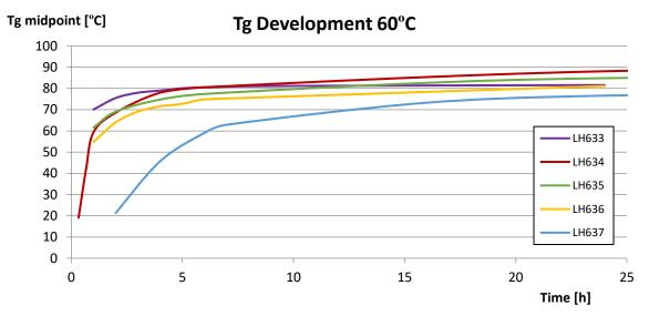
Measuring conditions: DSC-measuring heat rate: 20°C/min, sample mass 10-20 mg
