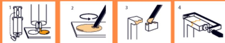
1 Snap off the resealable cap from between the syringe plungers and break off the end seal. Depress the plunger to dispense equal amounts of both components onto a clean disposable surface. Re-fit the cap to close the nozzle.
