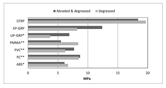
(\*): UP-GRP, ABS, substrate failure observed when abraded and degreased. (\*\*) : PMMA, PVC, PC, substrate failure observed in all conditions.
