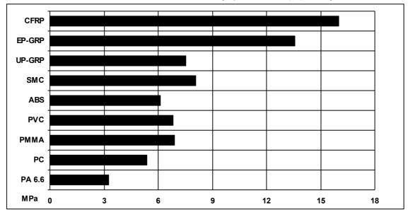
Average lap shear strengths of typical plastic-to-plastic joints (ISO 4587) (typical average values)
