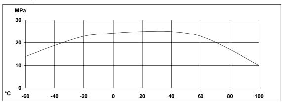
Roller peel test (ISO 4578)
